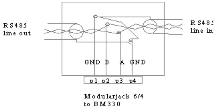
The cable for a direct connection of a BM330-1 to a 485 converter is shown below. The modular contact is seen from contact side.
