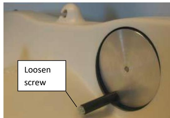
3: To dismantle the cover, loosen the four screws holding the cover and lift the cover off.
