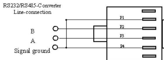
We recommend twisted pair cable with shield and return wire, e.g. type Alpha Wire 5471C. The return wire and the shield shall be connected to p1, p4 (GND) in every junction box.
