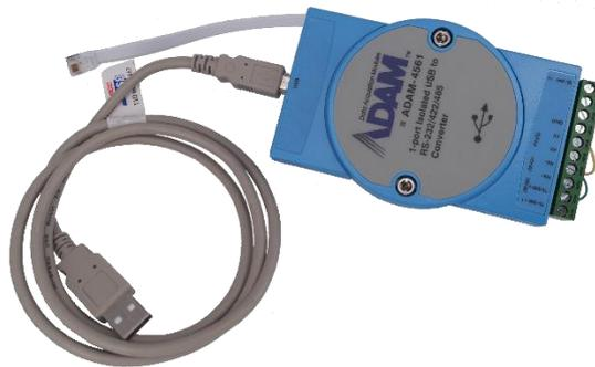
*Figure 1 Cable kit and adapter for communication with RS485 between Biomixer and PC.*
