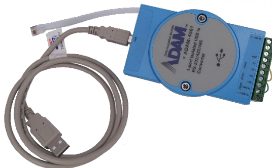
Cable kit and adapter for communication with RS485 between Biomixer and PC.
